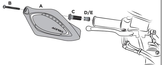
**Insert the screw (B) in the handguard (A), tighten it to the handlebar using the expander (C) and insert (D/E).**
