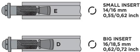
**Insert the correct expander nut (D or E) according to the handlebars' internal diameter.**
