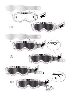
Maintenance: replace damaged tear-off immediately
